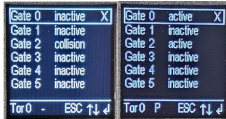
Figure 9-2 Gate inactive, collision / Gate active
