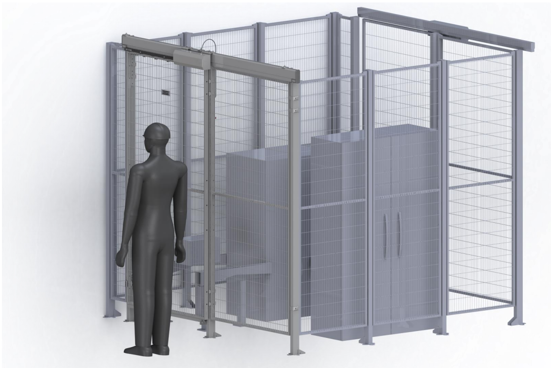
Figure 2-1 Single Sliding Door assembly with Power Door Single Rail PLC 24V
